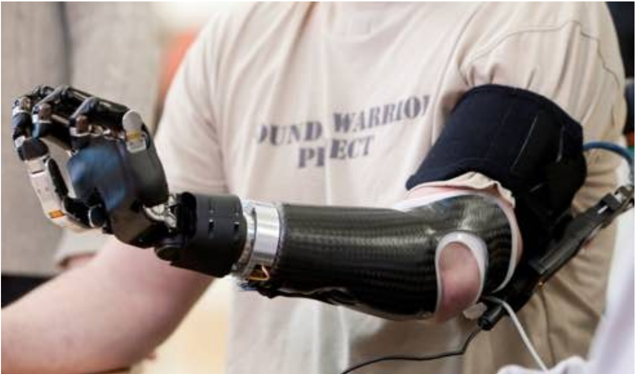
Fig. 3 Prosthesis controlled by brain waves.
